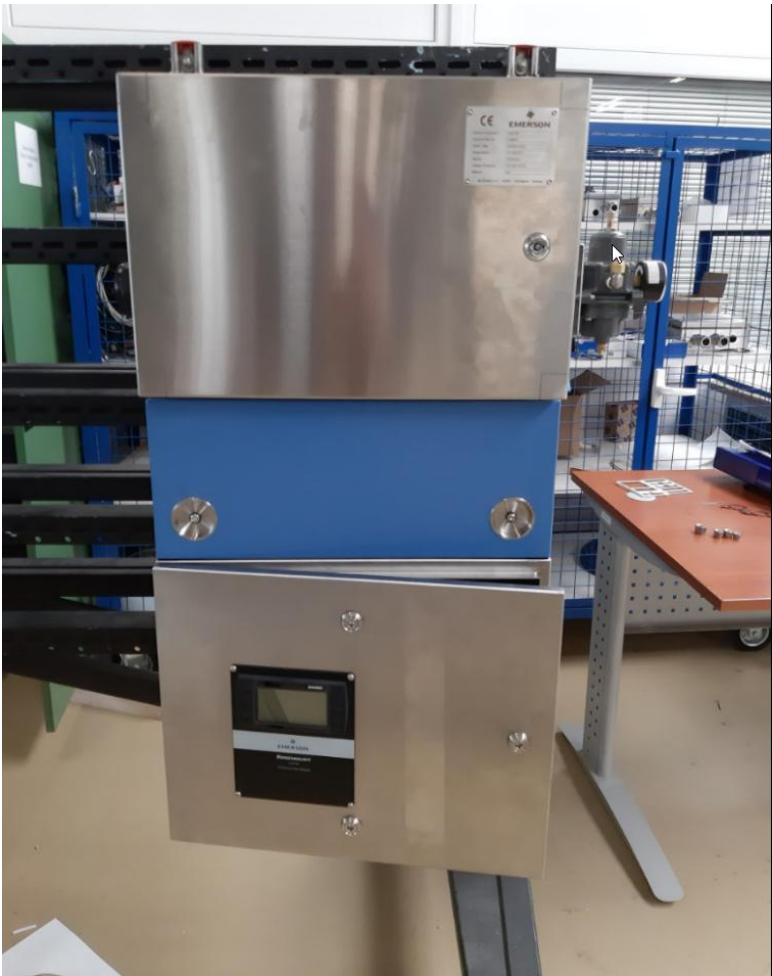
3 boxes solution (Sample system, Analyzer Cell & Analyzer Electronic)
